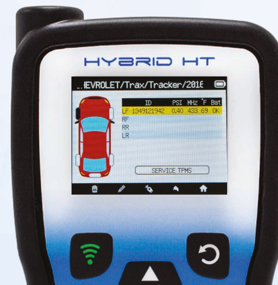
The tool will display the sensor's ID, battery status and frequency besides the tyre's pressure and temperature
